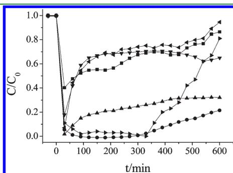
**Figure 7.** Breakthrough curves of elemental mercury capture by  $(\text{Fe}_2\text{Ti})_{0.8}\text{O}_4$ :  $\blacksquare$ , 200 °C;  $\bullet$ , 250 °C;  $\blacktriangle$ , 300 °C;  $\blacktriangledown$ , 350 °C; (left-facing triangle), 400 °C; (right-facing triangle), 250 °C with  $\text{SO}_2$ .
