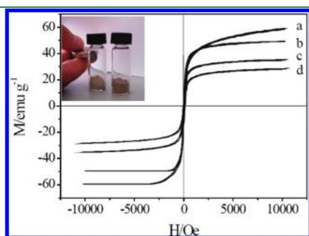
**Figure 6.** Magnetization characteristics of synthesized  $(\text{Fe}_{3-x}\text{Ti}_x)_{1-\delta}\text{O}_4$ : (a)  $x = 0$ ; (b)  $x = 0.3$ ; (c)  $x = 0.7$ ; (d)  $x = 1$ . The insert shows the result of separating  $(\text{Fe}_2\text{Ti})_{0.8}\text{O}_4$  from the fly ash.
