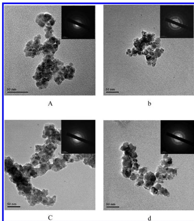
**Figure 3.** TEM images of synthesized  $(\text{Fe}_{3-x}\text{Ti}_x)_{1-\delta}\text{O}_4$ : (a)  $x = 0$ ; (b)  $x = 0.3$ ; (c)  $x = 0.7$ ; (d)  $x = 1$ . The insets show the selected area electron diffraction patterns of the nanoparticles.
